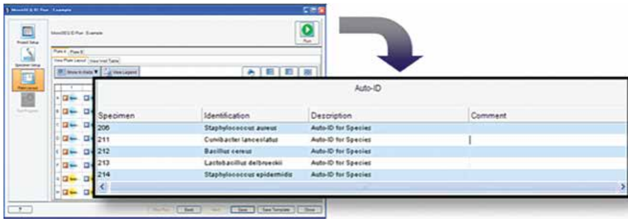
Figure 6. The Auto-ID feature of MicroSEQ® ID analysis software allows rapid identification of multiple specimens based on a predetermined set of acceptance criteria.
